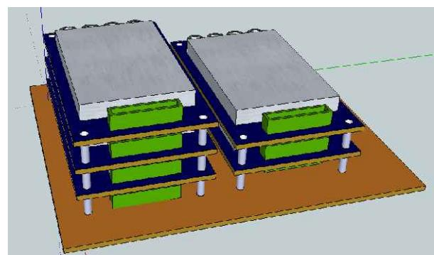
The **SmartBrick** modules are driven by a host system (microcontroller, DSP or PC, either embedded or remote) through the patented ultra-flexible **SmartBus** interface, compatible with USB, I2C, SPI or UART links. Open source software libraries provides an easy interface with any user-developped application in virtually any langage : Labview, C, C++, C#, Visual Basic, Matlab/Scilab, etc.
