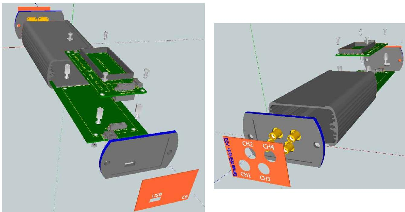
The **SmartBrick** module is fixed on the XS motherboard with four sets of spacers, washers, nuts and screws.
