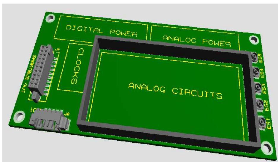
Mechanical fixing is done through four 2mm screws and spaces, insuring high vibration immunity.
