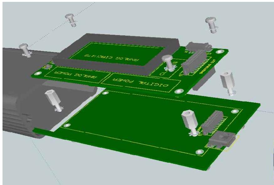
When assembled the XS motherboard + module assembly slides inside the enclosure and allows access to USB and analog connectors. These connectors are routed to front panel connectors through SMA to UFL jumpers (1 to 4) :
