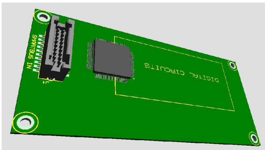
On the top side each module has a mating **SmartBus** stacking connector, which allows to stack several modules transparently. The top side has also a shielded enclosure which includes all sensitive mixed signal electronics. Analog I/Os are done through 1 to 5 subminiature UFL connectors. Lastly a dedicated connector allows factory operations.
