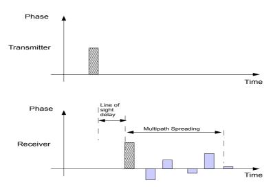
This induces two problems as the successive bursts are summed by the receiving antenna: fading (when the echoes are out of phase with each other, giving destructive or constructive interferences), and inter-symbol interference (when the duration of a binary bit is shorter than the time between the first and the last echoes).
