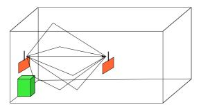
In the time-domain, when a short RF burst is transmitted by the first node this burst is received several times by the destination node, one time through each spatial path. Each reception is associated with a given attenuation and delay (corresponding also to a phase shift).
