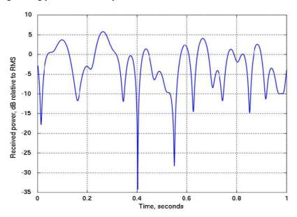
When one of the nodes is moved this plot shows the presence of deep fading situations, with variations usually in the 10dB to 15dB range but with occasional 30dB or more attenuations. Distance between peaks and valleys is roughly half a wavelength (giving 6,25cm at 2,4GHz), as to move from a signal in phase to a signal out of phase is equivalent to increasing the path length by half a wavelength.
