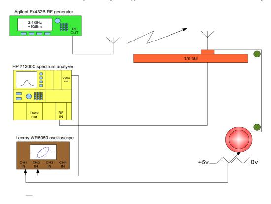
An Agilent E4432B RF generator drives a fixed dipole antenna with a 10mW 2,4GHz CW signal. This signal is received by a vertical monopole antenna, fixed on a ground plane sliding on a 1m-long aluminium rail. The line of sight (LOS) distance between the two antennas is 20cm to 1,20m (6 times farer), giving a theoretical attenuation of 15dB from one end to the other.
