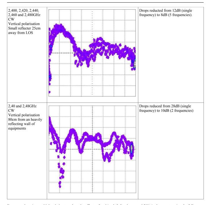
Frequency hopping could then helps to reduce the effects of multipath fading by around 50% in these tests, using the full 80MHz ISM bandwidth available at 2,4GHz. However as soon as the hopping band is reduced then the improvement is far lower.
