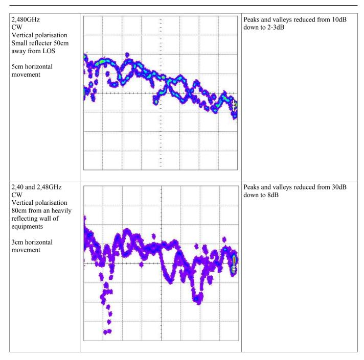
As expected spatial diversity is a very efficient way to minimize the effects of multipath fading. Best results were achieved with antennas separation of 3 to 5cm, corresponding to a quarter to a half wavelength at 2,4GHz.
